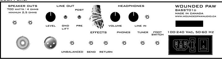
**Speaker Outputs:** Two 1/4" jacks and one Speakon jack all wired in parallel to connect to speaker cabinets. The absolute minimum load is 2.5 ohms but 4 ohms is recommended. The output power is 700 watts at 4 ohms or 350 watts at 8 ohms.
